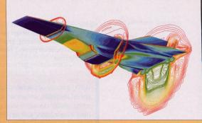
The underbody of the X-43 serves as inlet and exhaust nozzle, so models for propulsion, aerodynamics, and structures couple into a meta-model of huge dimensionality.
